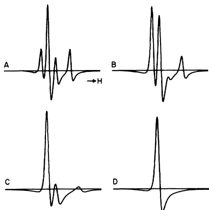
FIG. 2. ESR spectrum with hyperfine interaction as the exchange increases from weak to strong. g_s=2.033 , g_d=2.013 , 1/\gamma T_{sl}=1/\gamma T_{dl}=10 G, \delta_e/\delta=0.01 , \chi_r^0=1 , \chi_r^0(1)=1 , A_{hf}=60 G, I=1 , and A: \alpha\chi_s^0=-0.0002 ; B: \alpha\chi_s^0=-0.005 ; C: \alpha\chi_s^0=-0.01 ; D: \alpha\chi_s^0=-0.02 . The horizontal sweep range is 400 G. The signals are normalized the same peak-to-peak height.
